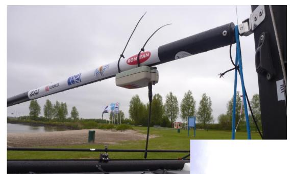
Place: On underside of the boom as pictured (must be clear of vange). Mounting material: 2 cable ties. Antenna to the bow of the boat. Do not bend antenna.
